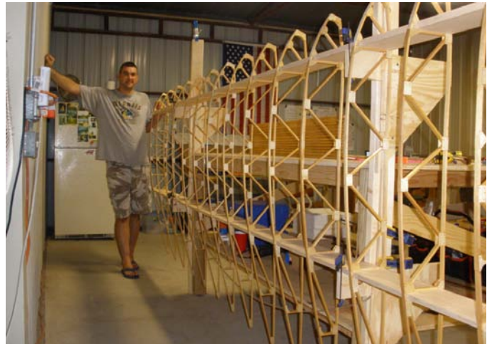
Ribs on the spars... on the wing jig.
