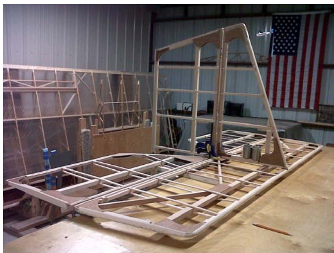
Empennage completed and hinges in place.
